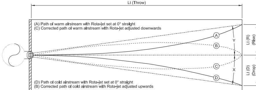
X = Downward angle of Rota-jet to overcome rise of warm air (maximum angle 30°)
